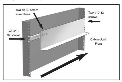
1. Affix the extension brackets to the main rail using the #8-32 screw/washer/nut assemblies. Adjust to the correct length for the cabinet depth being used.
